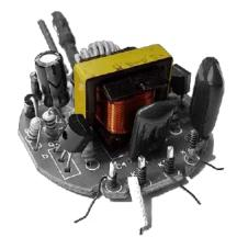
CFL power supply with desired transformer.
