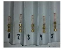
**FIG 6)** Aim to cut serrations or spool shapes into the pin.
