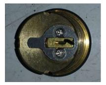
FIG 4) Remove the retainer
